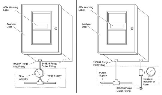
Components in dashed line are supplied by customer.
